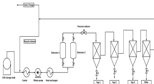
Fig. 1: Schematic for Supercritical Fluid pilot plant
