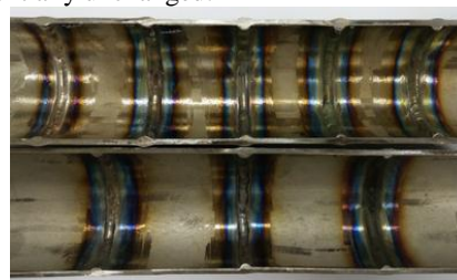
Fig. 1 The effective of % oxygen various to discoloration
