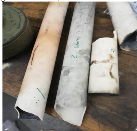
Fig 2: Alumina and alumina silicate tubes that suffered chemical attack and thermal shock
