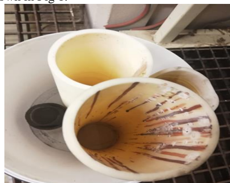
Fig 1: Alumina tubes, cracked due to thermal shock
