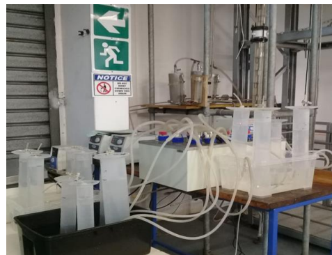
Fig. 2: Biochemical potential set-up at a mesophilic temperature of 40°C
