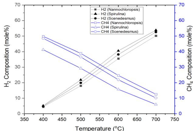
Fig. 2. Effect of temperature on H<sub>2</sub> and CH<sub>4</sub> gas composition (pressure: 30 MPa, biomass concentration: 10 wt%)
