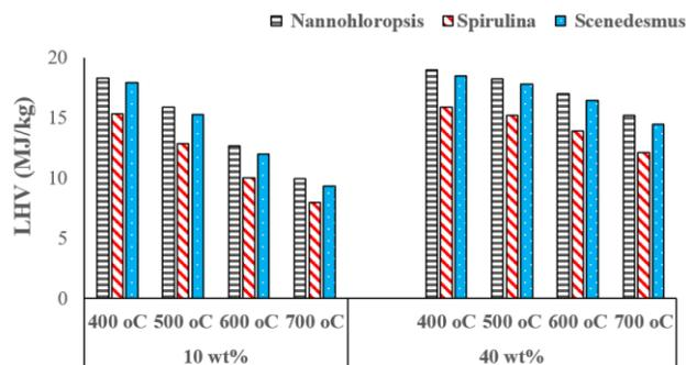
Fig. 6. Effect of temperature at different biomass concentration on the gas mixture lower heating value
