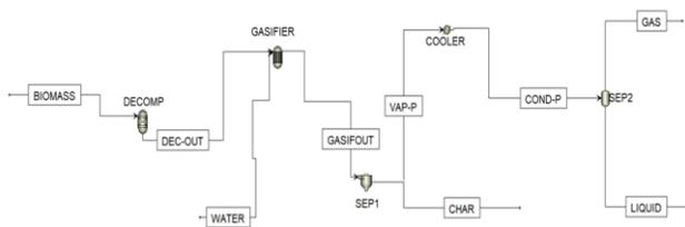
Fig 1. Aspen flow sheet for the supercritical water gasification process
