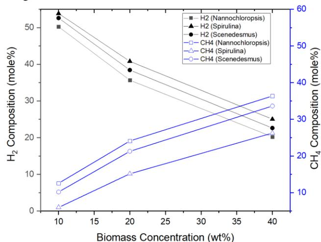
Fig. 4. Effect of biomass concentration on H<sub>2</sub> and CH<sub>4</sub> gas composition (pressure: 30 MPa, temperature: 700 °C)
