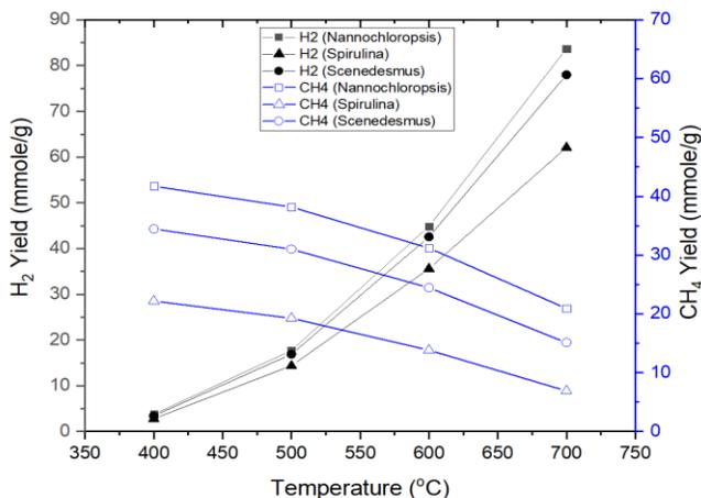
Fig. 3. Effect of temperature on H<sub>2</sub> and CH<sub>4</sub> gas yield (pressure: 30 MPa, biomass concentration: 10 wt%)
