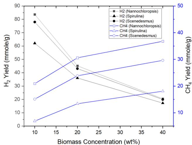
Fig. 5. Effect of biomass concentration on H<sub>2</sub> and CH<sub>4</sub> gas yield (pressure: 30 MPa, temperature: 700 °C)
