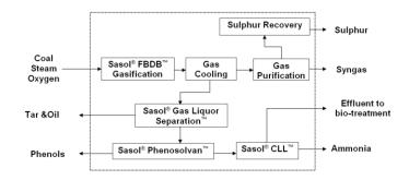
Fig. 2 Syngas production block flow diagram [23]
