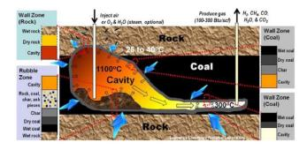
Fig. 3Typical cavity configuration of a mid-to-late stage of a linked vertical well module [30].
