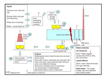
Fig. 4 Schematic diagram of the coke production process, indicating inputs, outputs and waste materials [38]
