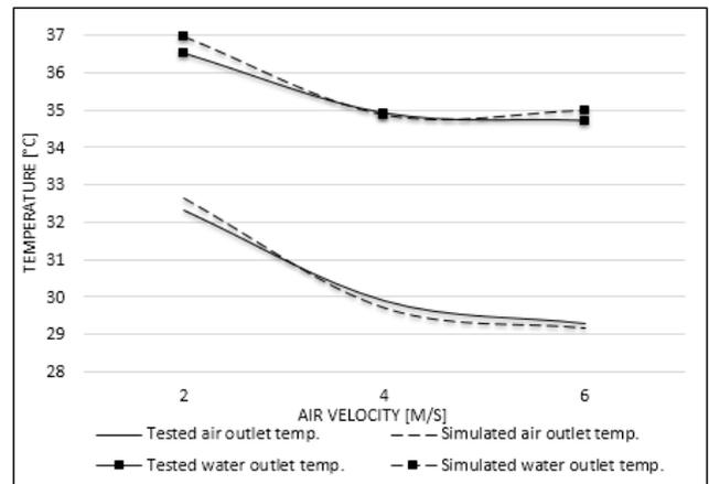
Fig 5 Simulated vs. tested: outlet temperatures 21 – 23 °C – 75 l/min
