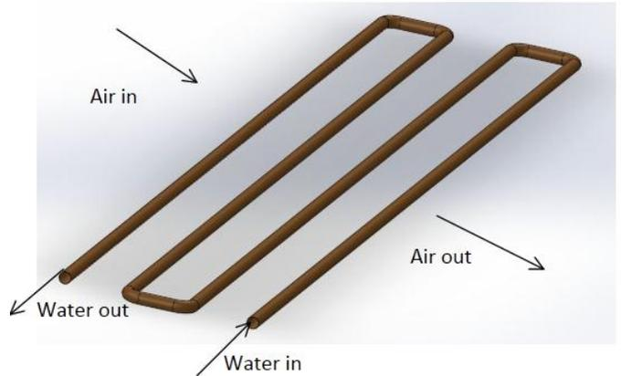
Fig 2 Simulated row of heat exchanger
