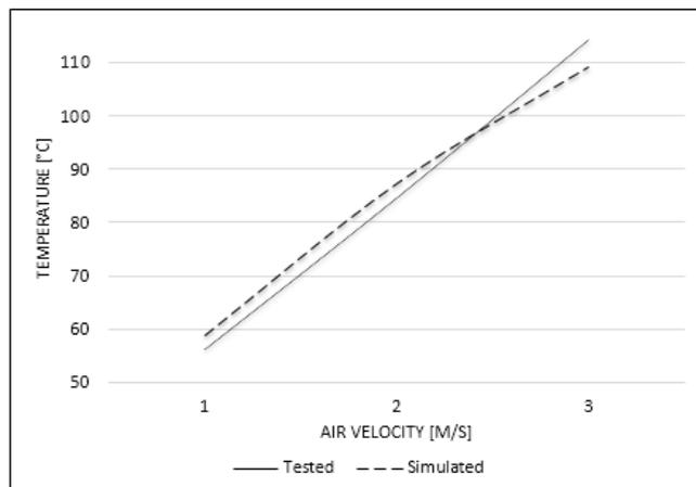
Fig 8 Convection heat transfer coefficient (air side), 21 – 23 °C, 75 l/min
