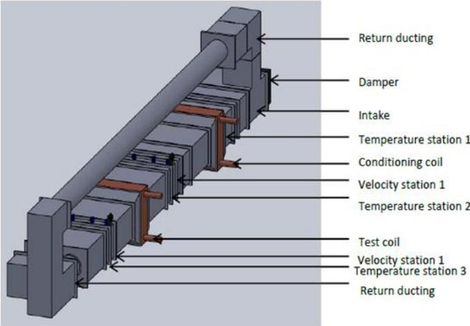
Fig 1 Layout of test bench [9].
