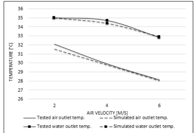
Fig 4 Simulated vs. tested: outlet temperatures 21 – 23 °C – 50 l/min
