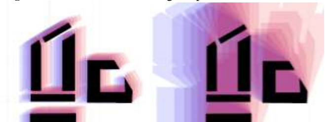
Fig. 5a Summer 9:00 to 15:00 Fig. 5b Winter 9:00 to 15:00 Fig. 5 Shadow Ranges In Summer and Winter
